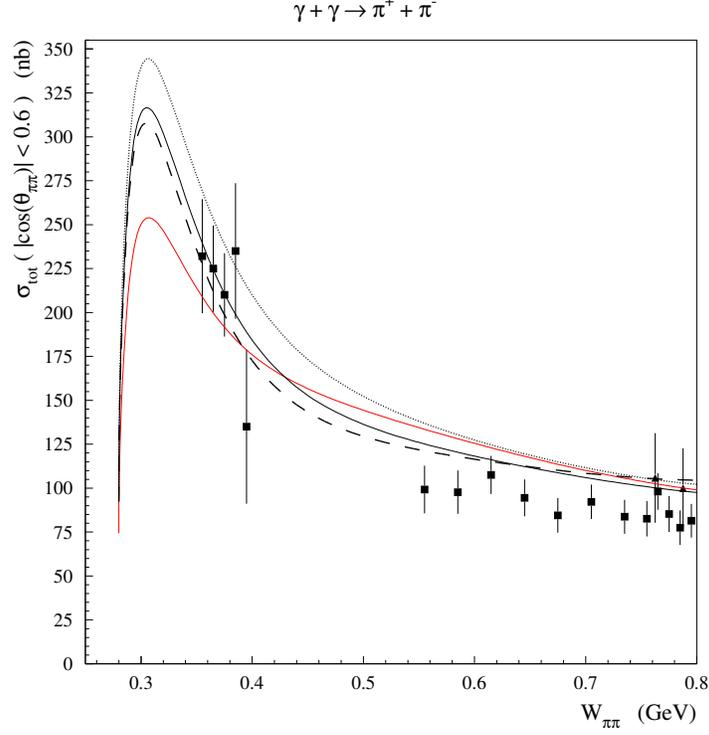
Figure 1:  $\gamma\gamma \rightarrow \pi^+\pi^-$  cross sections. Red curve: Born approx. (no polarizability effect); black solid: unsubtracted DR calculation with  $\alpha_\pi - \beta_\pi = 5.7$ ; dashed: subtracted DR with  $\alpha_\pi - \beta_\pi = 5.7$ ; dotted: subtracted DR with  $\alpha_\pi - \beta_\pi = 13.0$ .
