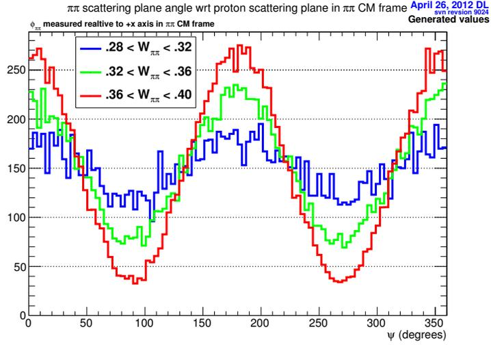
Figure 8: Histogram of  $\psi$  for Primakoff and  $\rho^0$  events. The blue curve is for events with  $0.28 < W_{\pi\pi} < 0.32$  GeV, green is for events with  $0.32 < W_{\pi\pi} < 0.36$  GeV, and red is for events with  $0.36 < W_{\pi\pi} < 0.40$  GeV.
