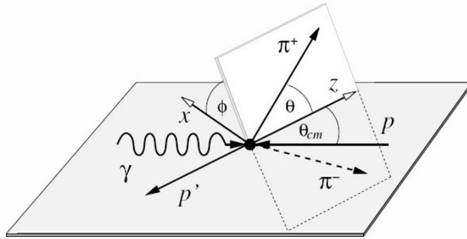
Figure 2: Diagram of the helicity frame for two pion photo-production on the nucleon
