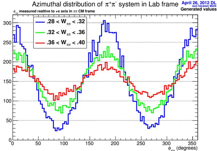
Figure 6: Histogram of  $\phi_{\pi\pi}$  for Primakoff and  $\rho^0$  events. The blue curve is for events with  $0.28 < W_{\pi\pi} < 0.32$  GeV, green is for events with  $0.32 < W_{\pi\pi} < 0.36$  GeV, and red is for events with  $0.36 < W_{\pi\pi} < 0.40$  GeV.
