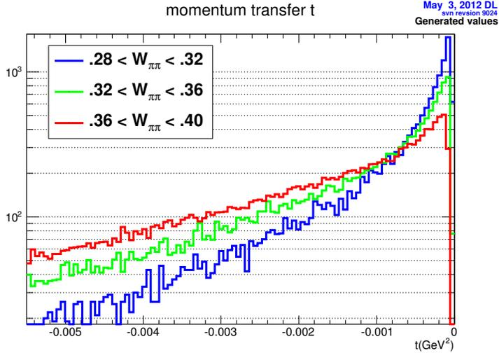
Figure 5: Histogram of  $t$  for Primakoff and  $\rho^0$  events. The blue curve is for events with  $0.28 < W_{\pi\pi} < 0.32$  GeV, green is for events with  $0.32 < W_{\pi\pi} < 0.36$  GeV, and red is for events with  $0.36 < W_{\pi\pi} < 0.40$  GeV.
