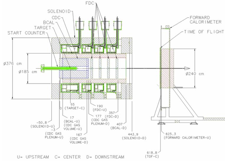
Figure 9: Diagram of the GlueX detector
