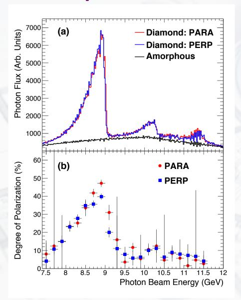
Coherent bremsstrahlung on diamond radiator. We tuned on a 9GeV photon energy for a 12GeV electron beam.
