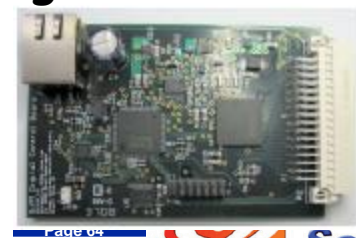
Digital Control Board
